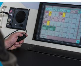
To provide access to both security domains (RED/BLACK) on a single operator position a secure switch is needed. A central component in RED/BLACK scenarios is the Frequentis iSAS which is a unique Secure Audio Switch that meets the Common Criteria recognition arrangement for components up to EAL4+ – NATO Secret.
